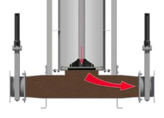
In the suction process, the inlet valve is open, the outlet valve is closed, the piston is in the bottom. The piston retracts and a negative pressure is formed in the piston pump and the slurry is sucked in.
